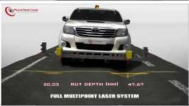
Minimum lasers required to calculate RUT is 5 lasers, recommended is 7.
